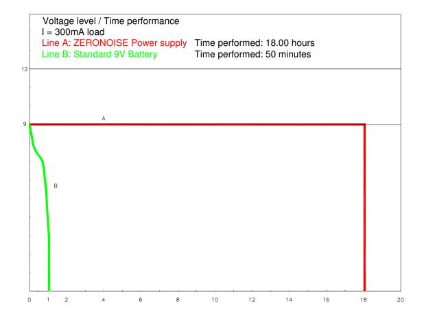
The above graph shows the huge difference in time of autonomy between a common 9V battery and the **ZeroNoise** power box: about 20 times more capacity and no degradation of output characteristics until the internal battery is completely discharge.
