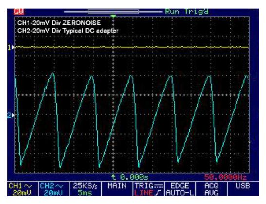
In the diagram (a) you can see the differences from a typical AC to DC adapter against **ZeroNoise**. The graphic shows that the DC output from the standard adapter introduces much more ripple noise into the signal as compared to the clean power produced by **ZeroNoise**.
