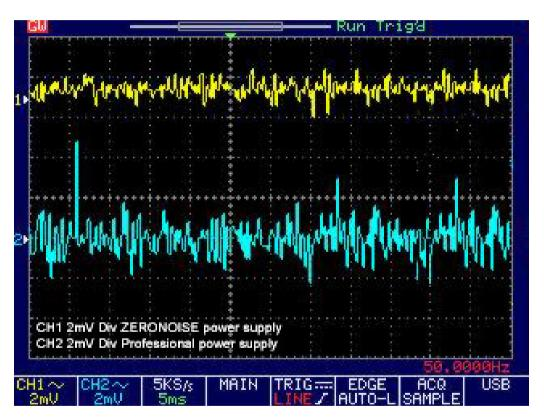
Graphic (b) represents the output produced by **ZeroNoise** compared with a professional DC power supply. The graphic shows that the standard DC professional power supply introduces significantly more ripple noise into the signal (approx twice as much) when compared to the **ZeroNoise** clean power.
